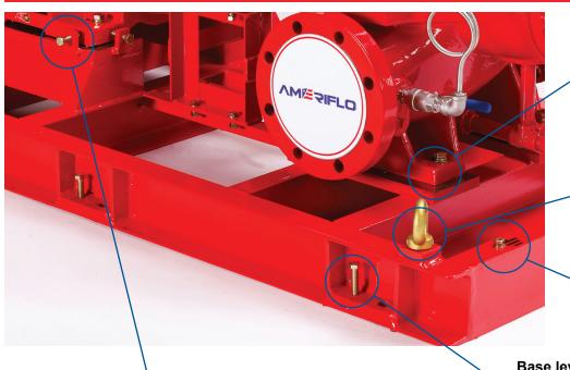
Milled pump & driver pads to ensure no soft foot present during installation
