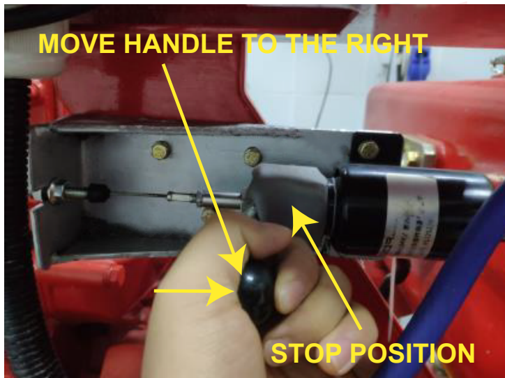
FIGURE 18 - EMERGENCY STOP USING BATTERY CONTACTORS
