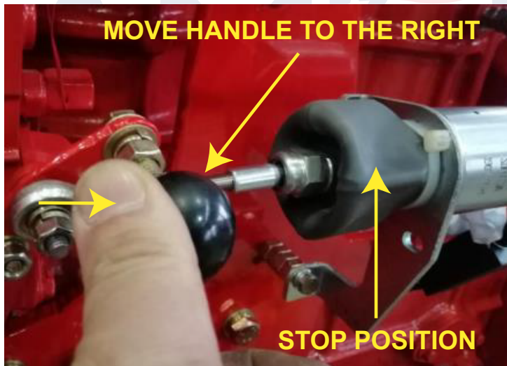
FIGURE 18 - EMERGENCY STOP USING BATTERY CONTACTORS
