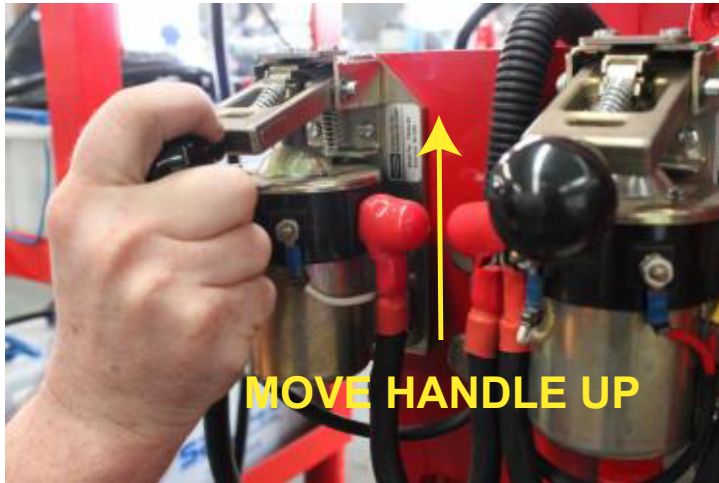
FIGURE 17 - EMERGENCY START USING BATTERY CONTACTORS
