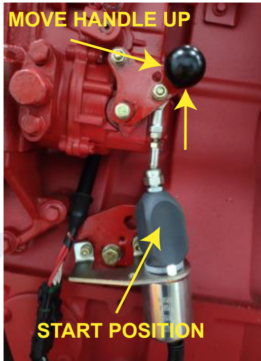
FIGURE 15 - SOLENOID RUN POSITION
