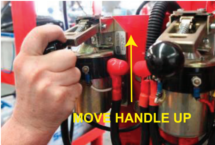
FIGURE 17 - EMERGENCY START USING BATTERY CONTACTORS
