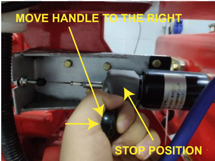
FIGURE 18 - EMERGENCY STOP USING BATTERY CONTACTORS
