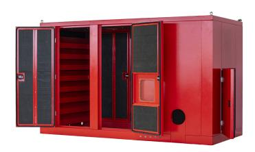
Mineral wool insulation is 4 inches thick and is applied to the entire interior of the enclosure. Unlike other enclosures provided by other diesel engine manufacturers, the diesel engine and pump are located within the enclosure. This type of installation also provides for sound attenuation of the pump assembly as well, providing a guieter installation.
